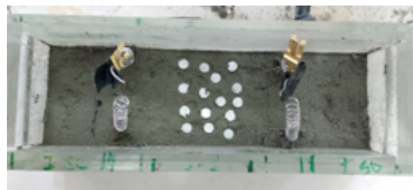
Figure 1: Cuts of an especial material used to create the anisotropic layer (Santos et al., 2017).
