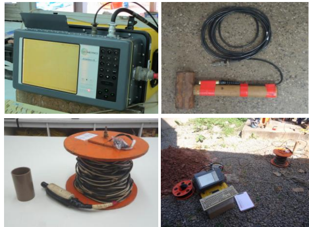
Figure 6 - Equipment used for the execution of PS test: seismograph (above on the left); 1.8-kg sledgehammer with trigger (above on the right); triaxial geophone hole with pneumatic system to fix in the hole (below on the left); equipment on the site (below on the right).
