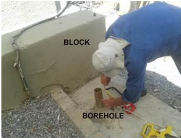
Figure 4 - Borehole for the PS test at 0.4-m distance from the block.
