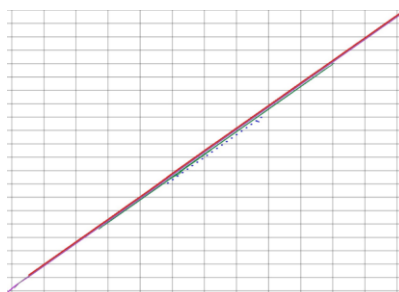
Figure 9 - 20 Wave Gliders (blue dots) deployed at a 300-m interval; the streamer vessel towing two streamers 2 km in length sailed parallel with the Wave Glider line.
