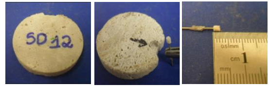
Figure 2: Preparation of a sub-sample for the acquisition of CT scans.
