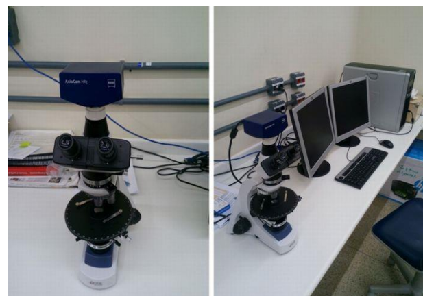
Figure 2: Microscope with coupled camera used to capture digital images.
