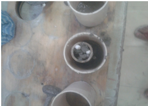
Figure 2: The use of the other pipe guaranteeing the location of the heterogeneities inside of the sample.
