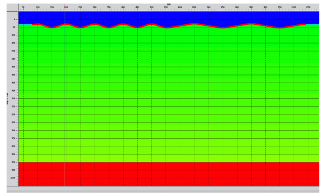
Figura 4: Example of the velocity field (Model 3) with the horizons of the LVL base.
