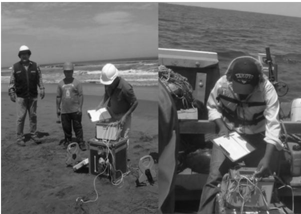
Figure 3 - Geophysical prospection by electrical tomography (right side continental prospecting, left side marine survey)
