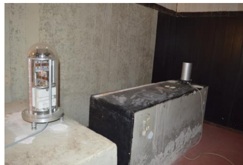
Figure 2 – TTB new variometers: DTU FGE (left) and GEOMAG-02M (right) sensors.
