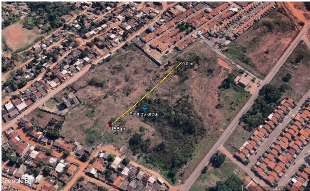
Figure 1. Location of the springs area in urban area of Cuiabá City, Mato Grosso State Brazil: The yellow line represents the ERT survey, red circles represents the initial and final profile and blue triangle is springs local area.
