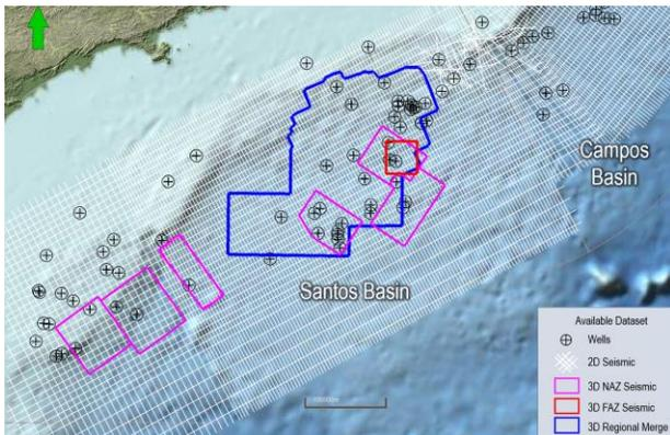
**Figure 3** - Available data set used in this study. (NAZ = narrow azimuth; FAZ = full azimuth)
