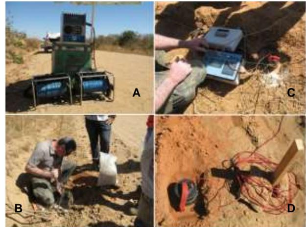
**Figure 5** – IP and Res data acquisition. A) VIP transmitter; B) steel electrode; C) *ElrecPro* receiver; D) non-polarizable electrodes.
