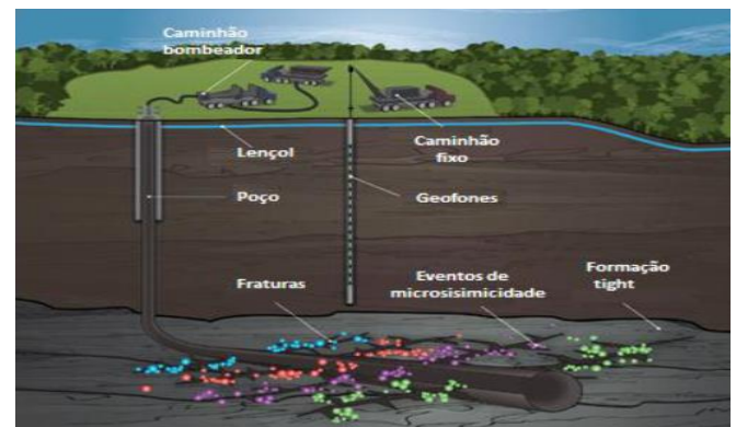
Figure 3: Microseismic monitoring of fracking (Oliveira, 2014).
