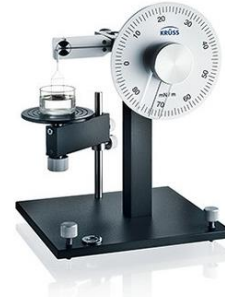
Figure 2: The K6 tensiometer. From: https://www.kruss-scientific.com/products/tensiometers/force-tensiometer-k6/
