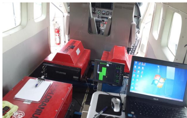
Figure 2 - Exploranium gamma-ray spectrometers, model GR-820, coupled to the interior of the aircraft.
