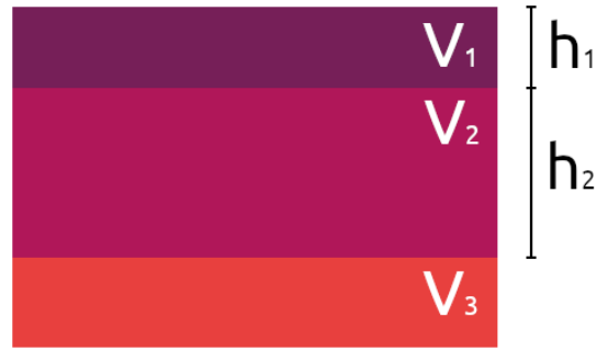
Figure 6: General 3-layered parallel-plane horizontal geologic model's seismic parameters scheme. Picture plotted with Matplotlib.
