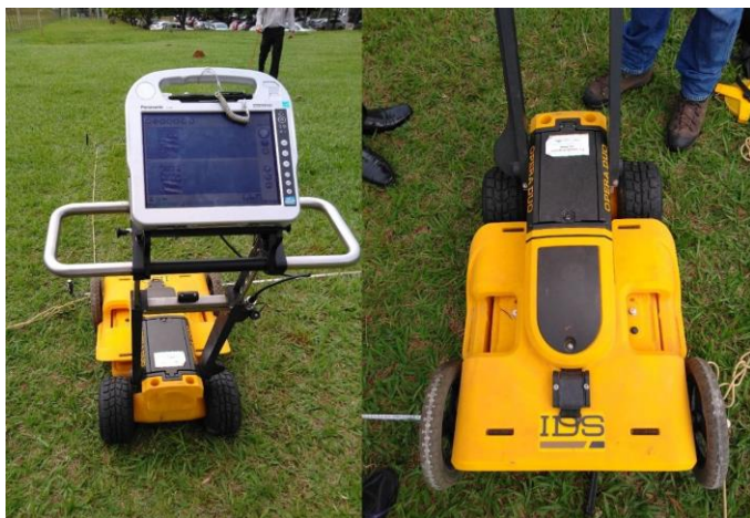
Figure 2 – Picture of the equipment Opera Duo (IDS Georadar) used in data capture.
