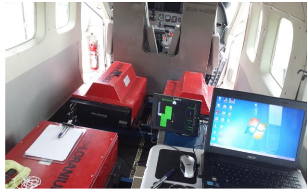
Figure 2 - Exploranium gamma-ray spectrometers, model GR-820, coupled to the interior of the aircraft
