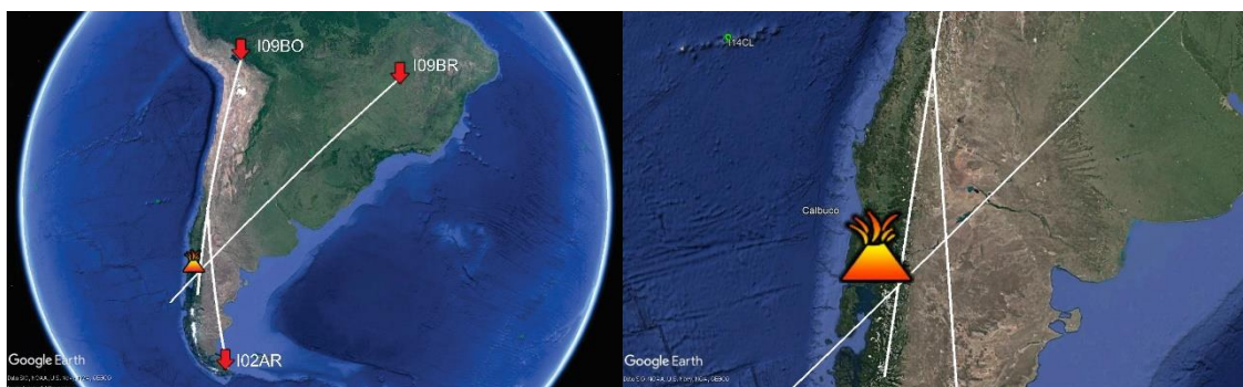
Figure 5 – Preliminary location of the Calbuco volcano eruption using the infrasonic data analysis
