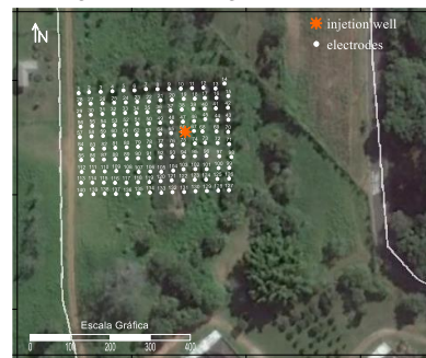
Figure 3 - 3D electrical imaging area with electrode distribution.
