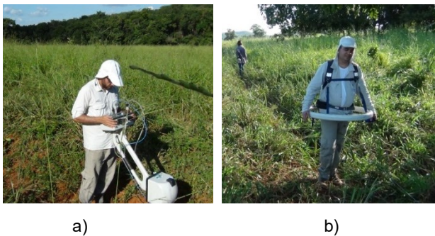
Figure 2: Details of the PROMIS-10 system: a) monitor and receiver-Rx; b) transmitting coil-Tx and batteries belt. Tx and Rx are connected by a reference cable.
