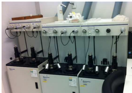
Figure 3 – Autopore IV 9520 from Micromeritics operating with a pressure limit of 66,000 psi
