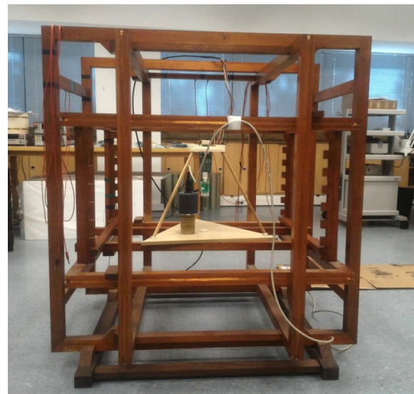
Figure 3 – Sensor in test on LDSM Helmholtz coil (source: LDSM).
