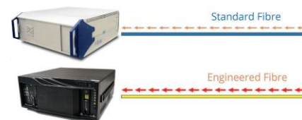
Figure 1. A cartoon depiction of how an engineered fiber reflects more laser light back to the interrogator than a standard fiber.
