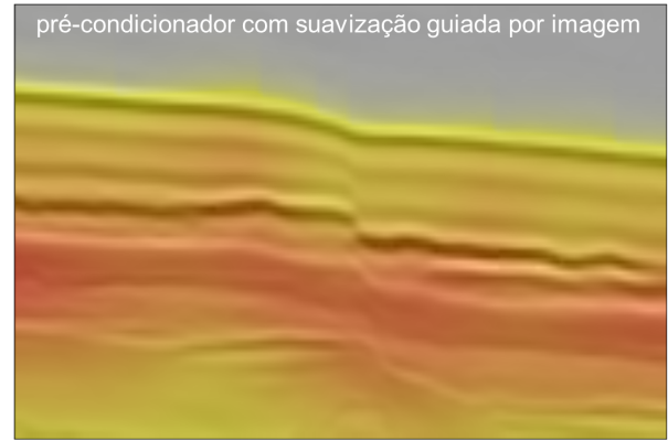
Figura 6: Model update with preconditioning by structural smoothing overlaid with the corresponding migrated image.
