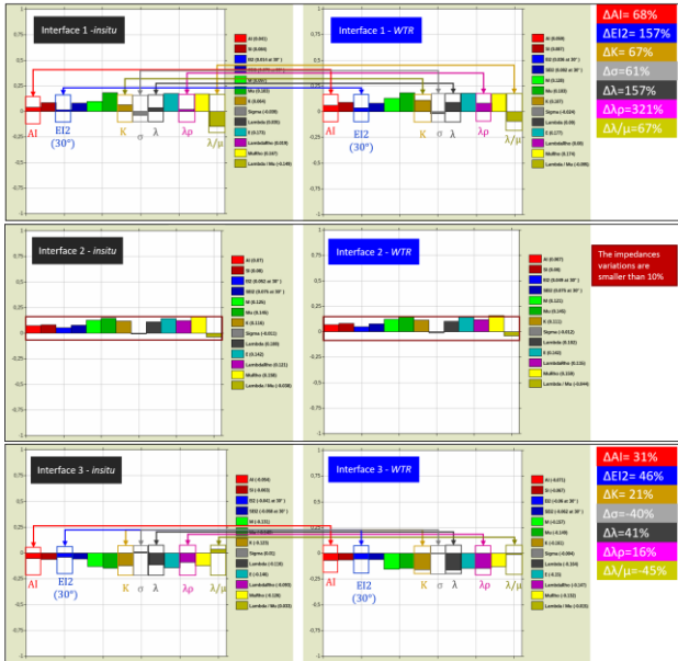
Figure 5 - Impedance contrast analysis between fluid scenarios per interfaces, showing the percentage variation of the scenarios.
