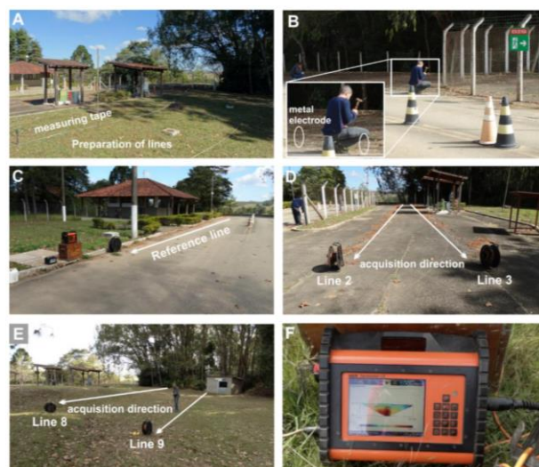
Figure 3 - Scheme for preparing the geophysical survey. A) Demarcation of the lines, B) Fixation of the metal electrodes. C) Assembly of the reference line (upstream), D) Acquisition lines in front of the supply pumps, E) Acquisition lines downstream of the filling station, F) Equipment with previous result.
