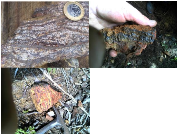
Figure 11- Looking clockwise: Typical magnetitic gneiss from the studied area with alternated bands of quartz and iron oxides (magnetite and hematite); Enriched altered gneiss with magnetite and other secondary iron bearing minerals such as goethite. Al-rich laterite.
