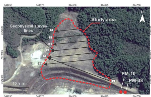
Figure 2 – Geophysical survey lines;; Location of monitoring wells PM-10 and PM-38.
