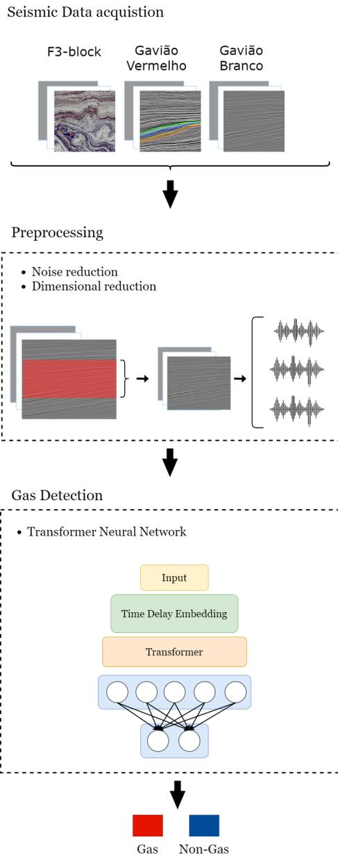
Figure 1: Flowchart of the method
