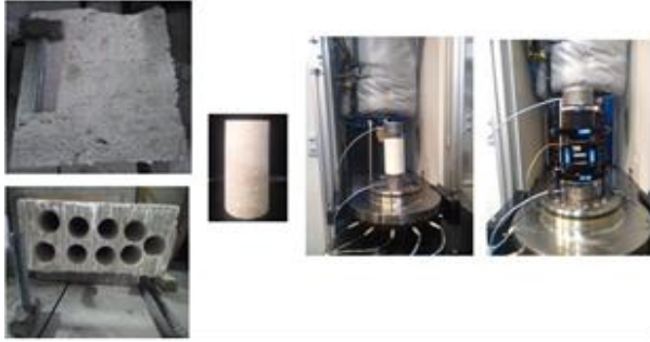
Figure 4: From left to right the roman travertine block, an extracted sample (plug), this same sample inside the compression press equipment and the once again the same sample, in which was added the strain gages.
