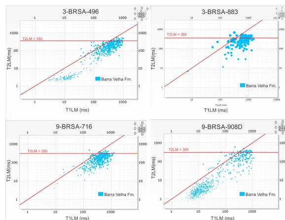
Figure 5: T1LM X T2LM crossplots show a horizontal trend between T2LM = 300 and 350 ms, indicating the predominance of bulk relaxation or vuggy porosity.
