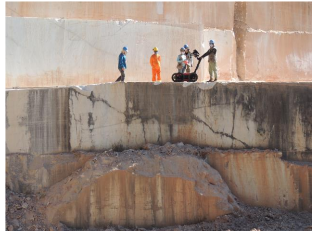
Figure 3 – GPR data acquisition.
