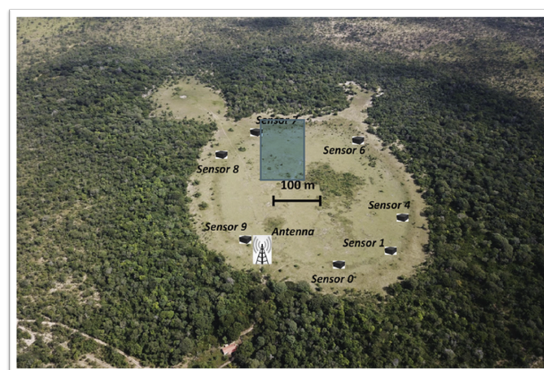
Fig 4. Location of H 2 monitoring in a circular depression of the São Francisco Basin (Brazil). H 2 sensors positions, and the data-transmitting antenna are shown (4).
