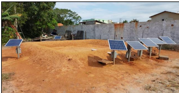
Figure 2 – Reduced-scale dam instrumented with microseismic stations powered by solar energy
