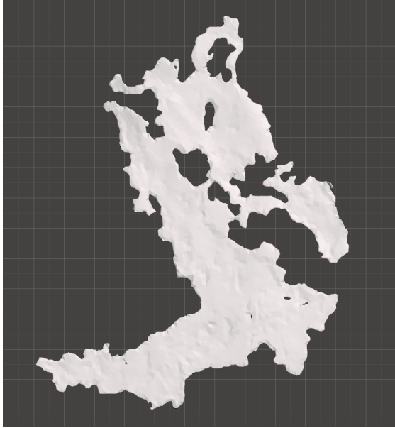
Figure 5 – The reservoir surface after point cloud filtering and mesh generation algorithm application. This geometry will be imported into the COMSOL software.
