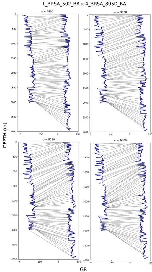
Figure 8 – Correlation lines between the well logs from 1-BRSA-502-BA and 4-BRSA-895D-BA, with different values of the restriction parameter  $\omega$ .
