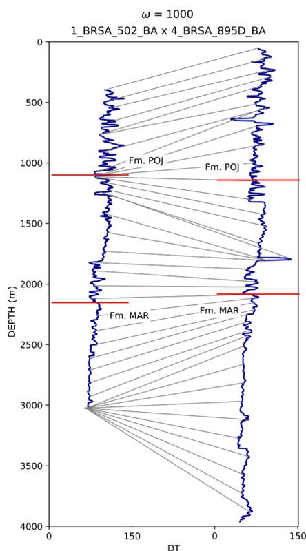
Figure 10 – Correlation lines obtained by the DTW algorithm between the seismic slowness logs of wells 1-BRSA-502-BA and 4-BRSA-895D-BA indicating which samples in depth correlate with each other, according to the alignment path obtained using the sonic log. The red lines highlight the patterns considered key in the correlation between the logs. The Sakoe-Chiba parameter adopted was 1000.
