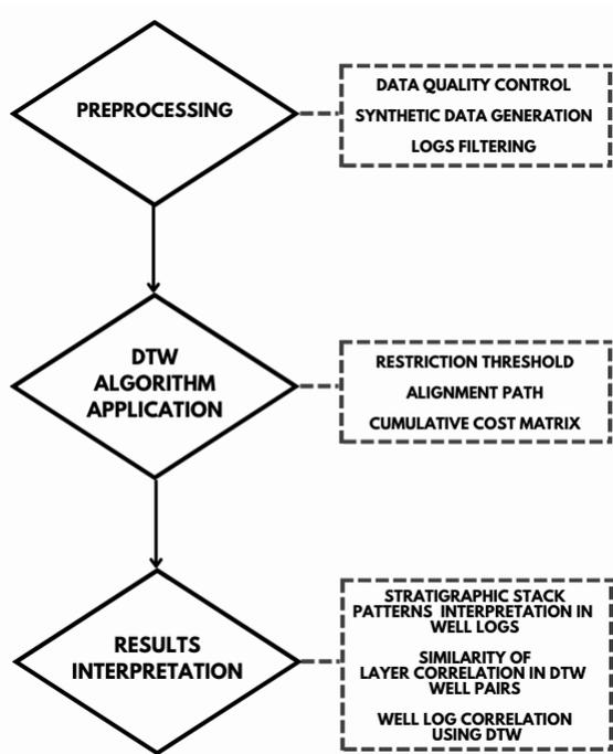
Figure 3 – Workflow employed to perform the well-log correlations using the Dynamic Time Warping Algorithm.
