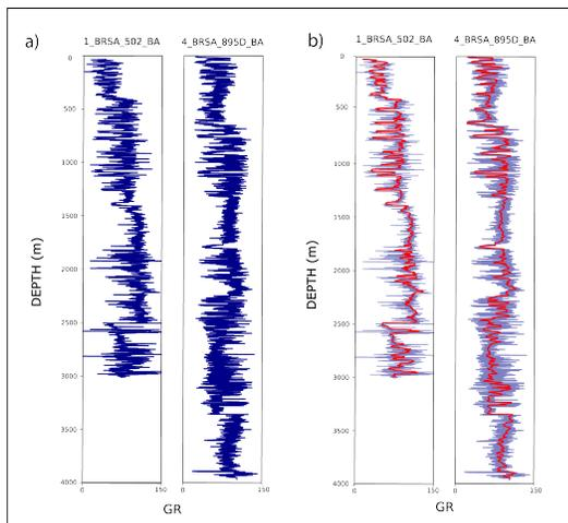
Figure 4 – Figure a) gamma-ray logs in wells 1-BRSA-502-BA and 4-BRSA-895D-BA without smoothing; b) shows the original curve (blue) and the smoothed measure (in red) after filtering using the 101-sample window median filter.
