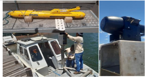
Figure 4 - A) Side-Scan Sonar B) Multibeam Echosounder C) Hydrographic vessel Stella VII docked during equipment setup.
