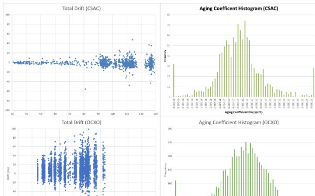
Figure 2 Comparison of Total Drift and Aging for a project acquired using nodes with CSAC's against a project acquired using nodes with crystal oscillators. For the project using crystal oscillators the aging coefficient was derived from first break analysis. While the total drift of the crystal oscillator is one order of magnitude higher than the CSAC, the aging characteristics of the two projects are very similar. The reason for this is that the crystal oscillator approach has much less control over the starting frequency. With both clock types the frequency is tuned to match the nominal clock frequency prior to deployment. However crystal oscillators are temperature dependent. See figure 2 detailing an experiment to measure the frequency change as a consequence of temperature. Frequency disciplining performed on the vessel will be imperfect
