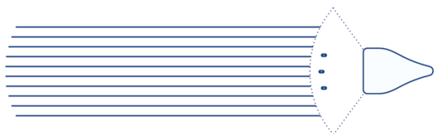
Figure 7 – High integrity ultra-high resolution P-cable configuration with a 10 x 6.25 m x 100 m streamer spread and a wide-tow triple source.
