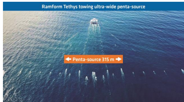
Figure 4 - Drone photo showing Ramform Tethys during a seismic programme in the Barents Sea in 2020. The seismic vessel is towing an ultra-wide penta source with 78.75 m source separation and 315 m total source spread width. The source separation is larger than the streamer separation (56.25 m).
