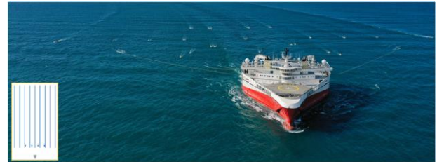
Figure 6 - Ramform Hyperion acquiring a high-resolution CCS development survey for the Northern Endurance Partnership offshore UK in 2022. The configuration consisted of 11 multisensor streamers with 50 m separation and a wide-tow quad source that was towed over the front end of the streamer spread. The resulting nominal acquisition bin size was 6.25 m x 6.25 m.
