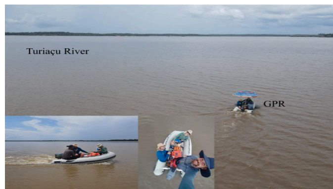
Figure 2: GPR data acquisition using a rubber boat on the Turiaçu River. Source: Porsani et al., 2023.
