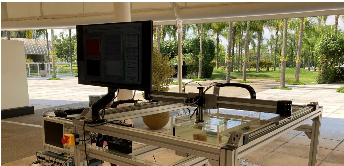
Figure 2: Final Prototype. This equipment is equipped with control over three axes (x, y, and z) and can analyze an area of 1000mm x 800mm. Furthermore, it allows the interchange of transducers with different frequencies.
