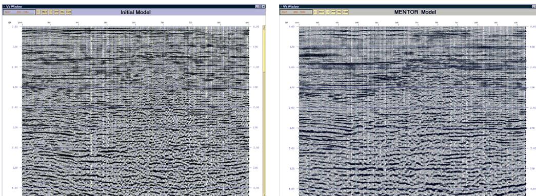
Comparison of prestack depth migration from offshore Australia using a) vertical updating and b) tomographic inversion
