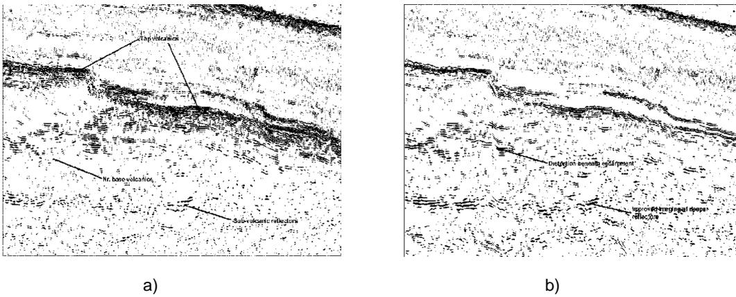
Comparison of sub-basalt imaging in the Shetland\_Faroes basin using a) 2D prestack time migration and b) 2D prestack depth migration.
