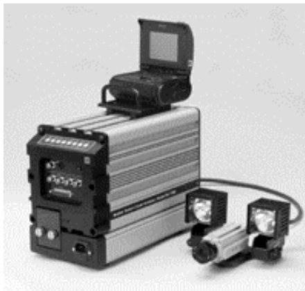
Fig. 1 – A high speed CCD-camera system (Kodak Motioncorder Analyser, Model SR-500).
