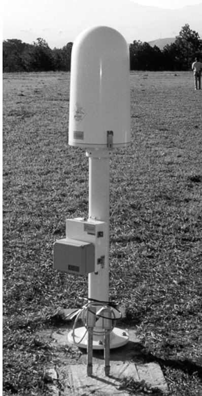
Fig. 2 – A sensor of Lightning Positioning and Tracking System installed in Cachoeira Paulista, SP, Brazil.
