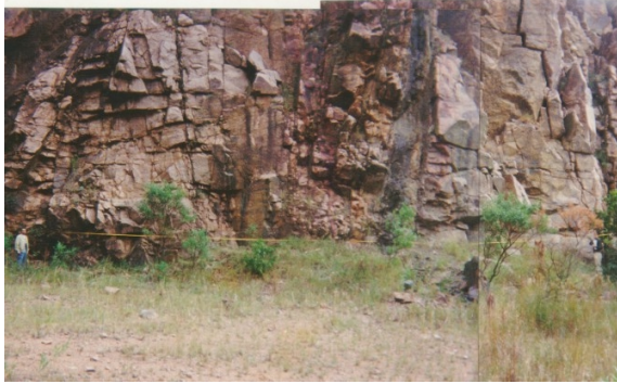
Figure 05 – Controlled photography of the the same granite-type dimension stone quarry as figure 03 and 04. Compare fracture sets showed in this photography and that defined in the radargram of figure 04.
