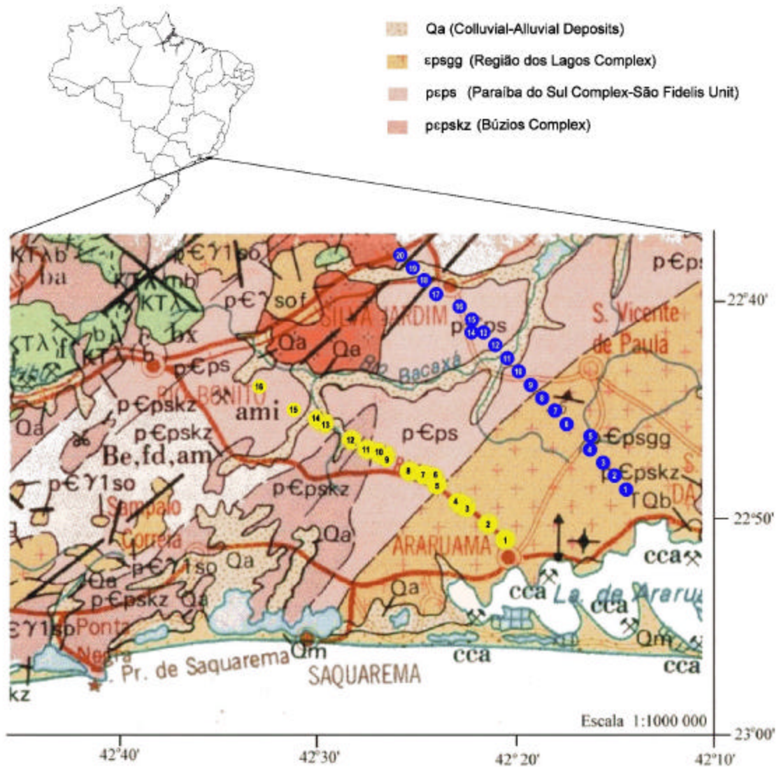
Fig. 1 – Geologic map and MT-TEM site locations. Profile 1 in yellow (Araruama - Rio Bonito profile). Profile 2 in blue (Iguaba - Silva Jardim profile).
