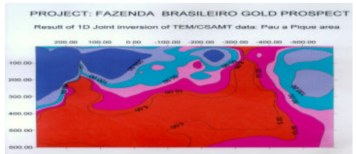
Figure 4 Joint TEM-CSAMT inversion model.
