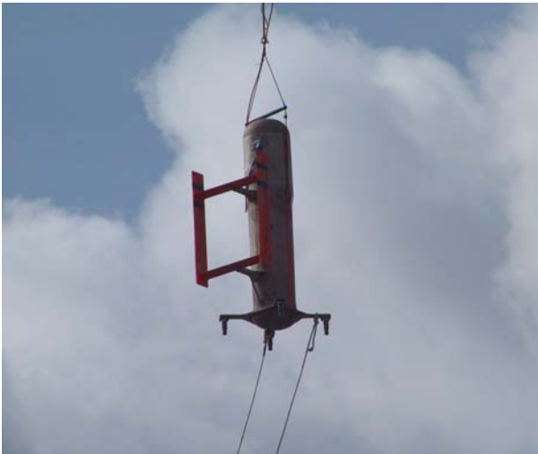
Figure 2. DRDC tow-body, containing the SQUID sensor and electronics, in flight.
