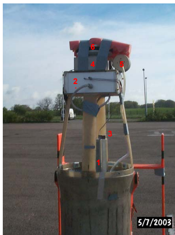
Figure 1. Electronics and sensors mounted on above the dewar: 1) SQUID controller electronics, 2) second electronics box, 3) accelerometer, 4) batteries, 5) pressure reference cell, 6) GPS antenna.
