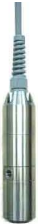
Figure 2 – Downhole fluorometer probe (max. diameter: 48 mm). This probe is equipped with two optics, one of which can be selected for turbidity measurements. The probe conveniently detects dye tracers in 2" boreholes to depths of 100 m.
