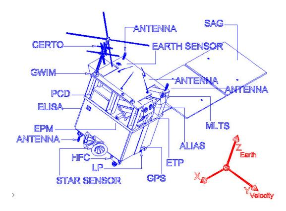
Fig. 1. Mechanical Design View of EQUARS satellite (preliminary).
